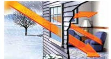
**Winter Energy Savings:** Low-E insulating glass reduces heat loss by reflecting warm air back into your home.
